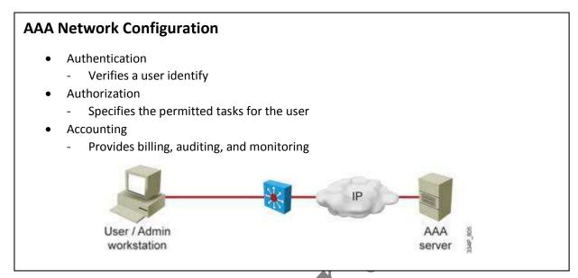
Authentication, authorization, and accounting (AAA) network security services provide the primary framework through which access control is set up on a switch. AAA is an architectural framework for configuring a set of three independent security functions in a consistent manner. AAA provides a modular way of performing these services. For purposes of this course, only authentication will be discussed.
