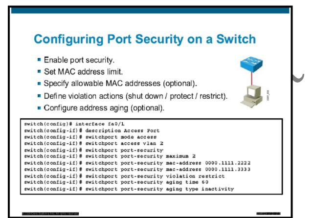
To configure port security so that switch port access is limited to a finite number and a specific set of enddevice MAC addresses, follow the steps in the table.
